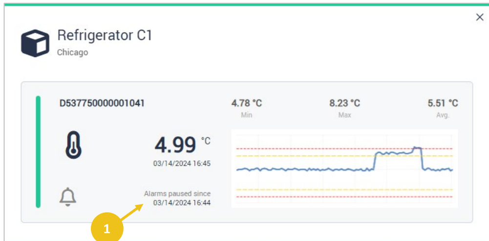
Figure 34 –Sensor details panel showing alarm pause is activated on the data logger
