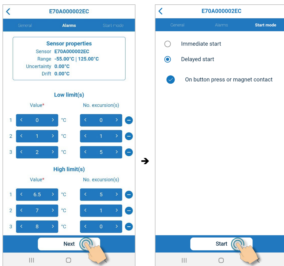
Starting data logging with high and low alarm limits
